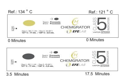
CHEMGRATOR integrating indicators are specially designed to integrate the effects of time, temperature and saturated steam in sterilization processes.
